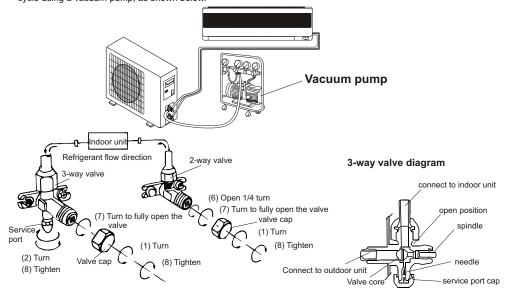
$\label{thm:local_problem} \textbf{Note: To protect the environment, be sure not to discharge the refrigerant to the air directly.}$
